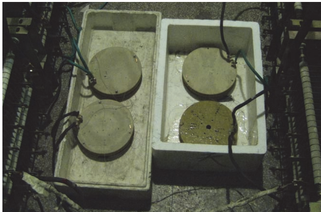
Fig. 24. Prototype SFCL and test circuitries.
